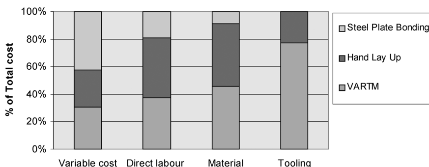
Figure 24. Initial project cost for repair of 6.4 m 2 of concrete girder using three different approaches.
